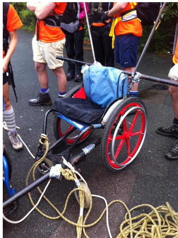
Extra wide push bars have to be lifted over gate posts.
