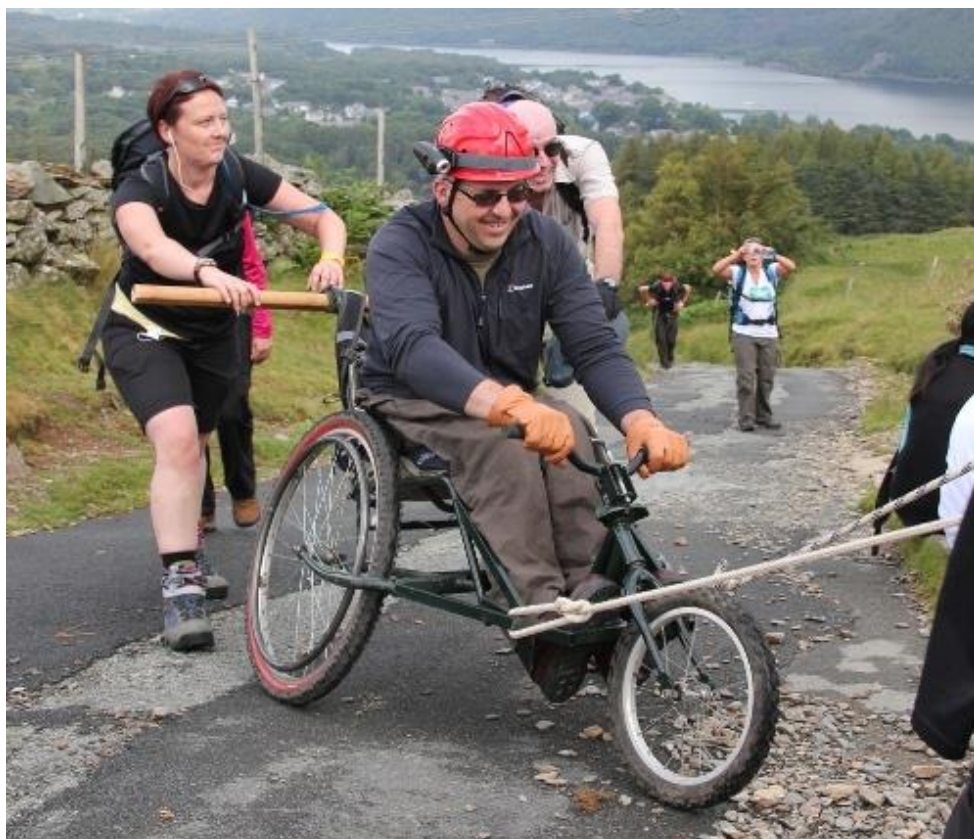
Fixed front wheel, SCI person well strapped in legs secured with straps.
