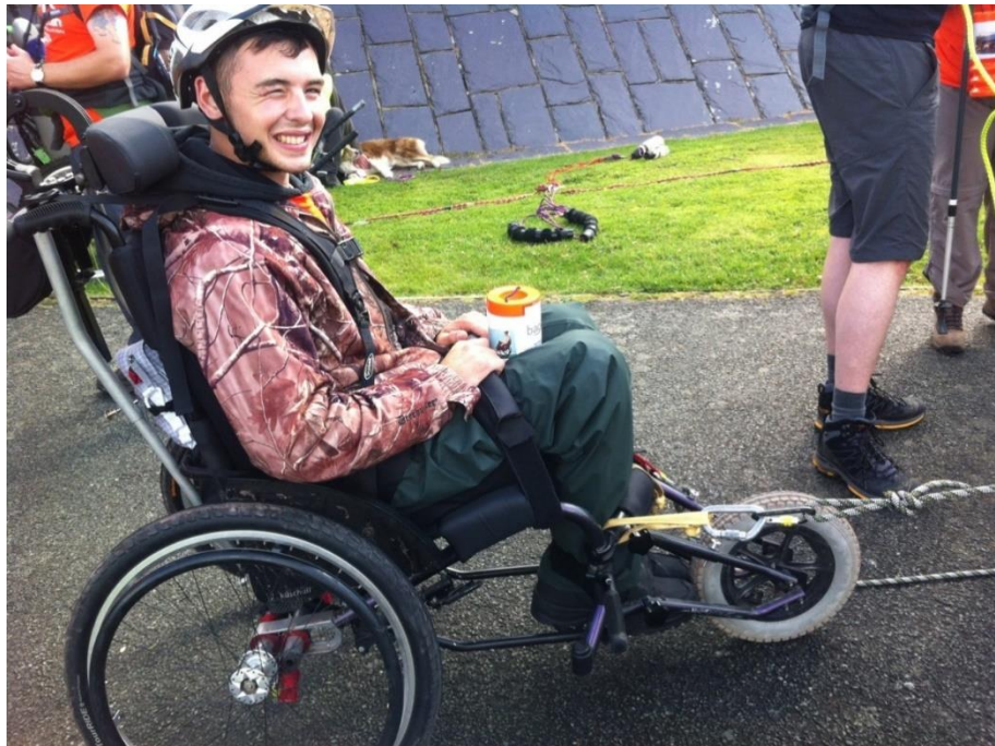
Fixed front wheel, SCI person well strapped in legs secured with straps.
