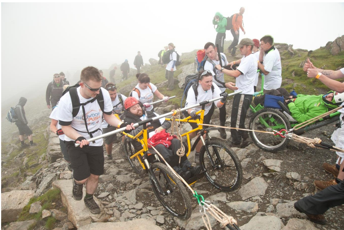
Big steerable 3 wheel design with wide bars for team members to use. Disc brakes on front wheels.
