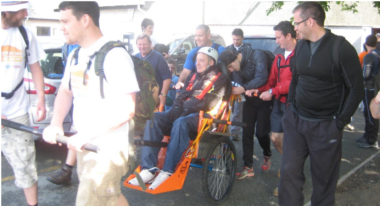
Foot plate with high sides, SCI team member is secured with shoulder and waist straps.
